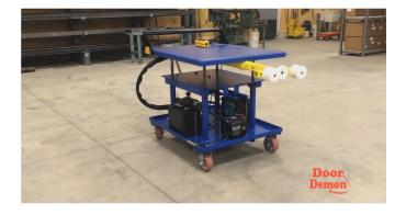
The Blue Roller Boxcar Plug Door Opener is a stand-alone unit designed to meet your needs where a forklift mounted unit doesn't fit. This design features safety, mobility, and adjustability in a compact and stable platform. This unit is small enough to store anywhere yet durable enough to remove the risk and hardship out of opening even the toughest, most damaged plug doors.
