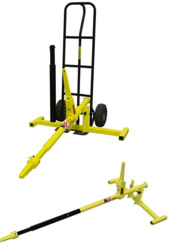
The Demon Stick is our manual, low-cost opener which can be carried or mounted to a two-wheel cart. Ideal for lower volume operations or as a backup unit, the Demon Stick allows the operator to get out from under the railcar, while putting the operator in a better position to open difficult gates. The reversible ratchet drive allows for easy direction change.
