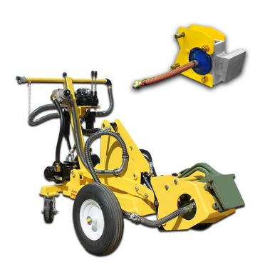
While railcar vibration is extremely important for unloading railcars quickly and safely, handling the vibrator or shaker is a difficult task, as they range in weight from 65 to 165 pounds. The patented\* Rhino Railcar Vibrator Lifter completely removes the danger of inserting and removing heavy railcar vibrators from the pockets of hopper cars.
