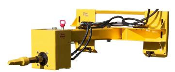
The Quick-Tach Hopper Gate Opener utilizes a universal mount quick attach plate allowing it to be easily mounted to most skid-steers or similar loading devices. This unit's hydraulic motor is powered by the hydraulic system of the skid steer or similar device via the auxiliary hydraulic ports. This makes the Quick-Tach a great solution where power options such as air and electric are not available.
