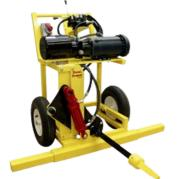
The AC Electric Two-Wheel Hopper Gate Opener is one of our most popular models. The powerful electric over hydraulic system provides enough continuous torque to open even the toughest railcar hopper gates.
