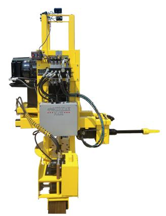
High volume unloading areas require the highest speed, efficiency, and obviously safety. Our new PowerDrive Multi-Position unit provides all of this, allowing the operator to control the unit from a comfortable position. This unit features our largest electric over hydraulic system. With simple hand controls or the optional remote transmitter, the operator can traverse the beam while adjusting drive bit height and position to fit any railcar.
